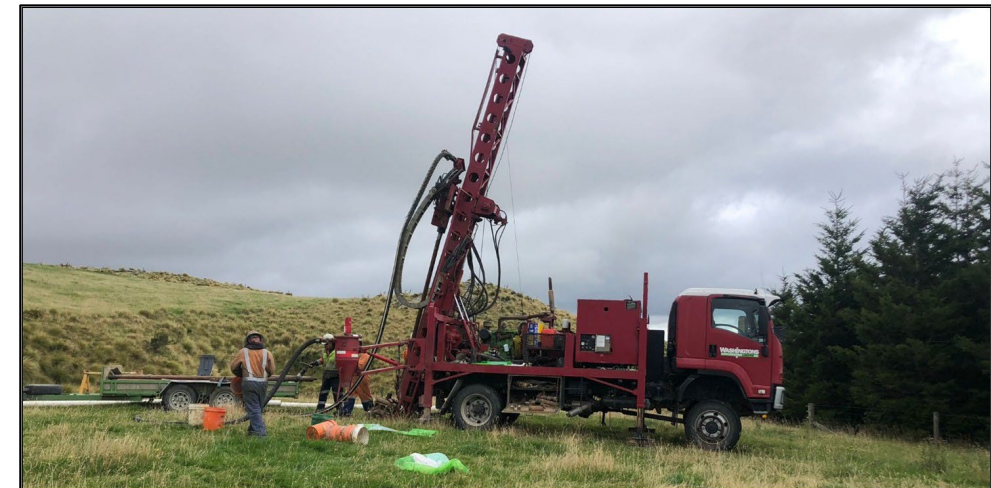
Dual-purpose (RC and diamond) drill rig deployed at the Lammerlaw, Central Otago region, New Zealand
