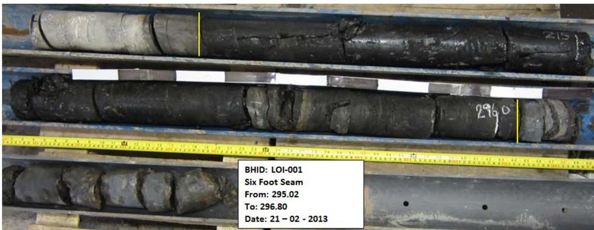
Figure 2: LOI-001 - Six Foot Coal Seam Core<sup>1</sup>
